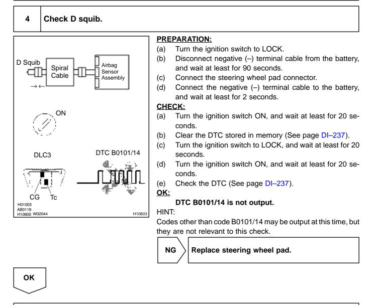
From results of above inspection, suspected part can now be considered normal. To make sure of this, use simulation method to check.
